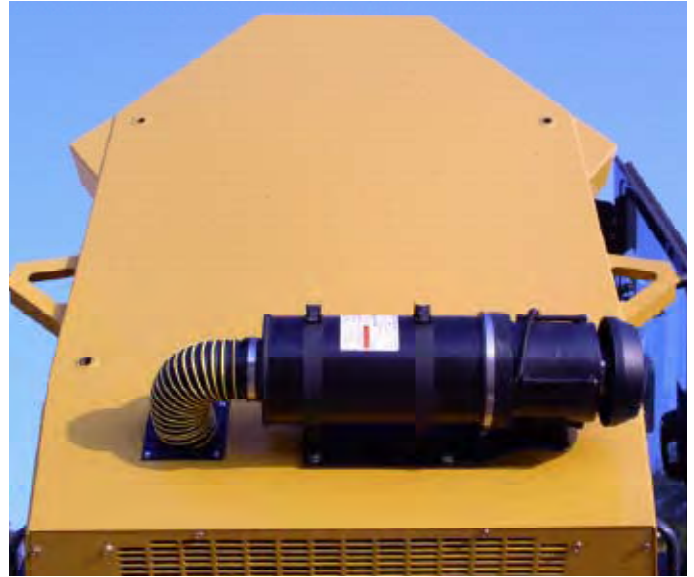
Figure 5: Gideon system installed on roof.
