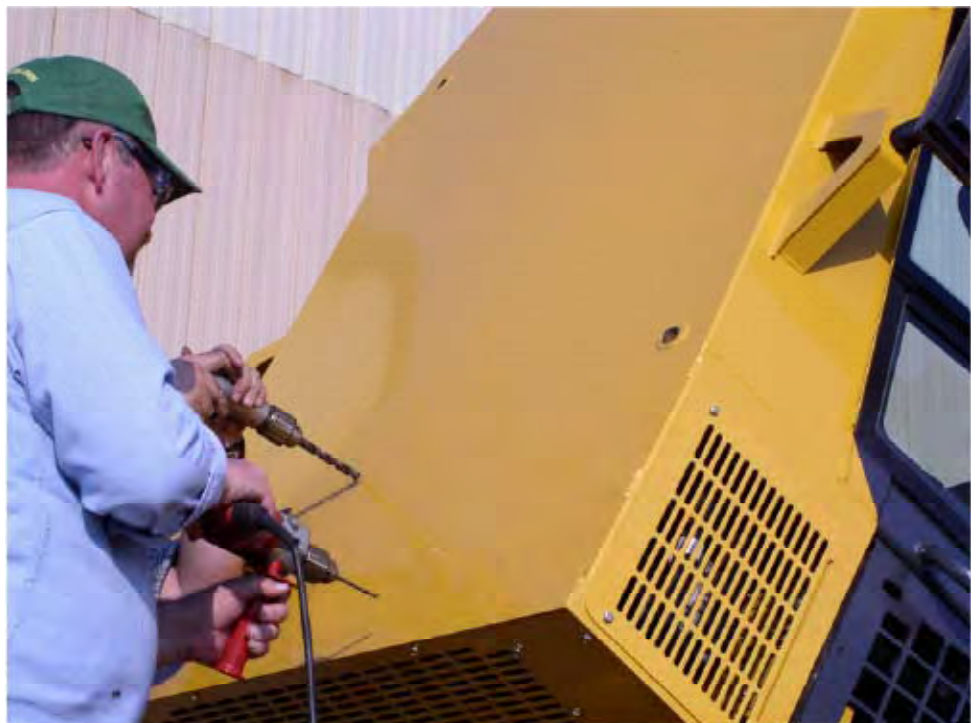
Figure 4: Locating and drilling mounting holes
