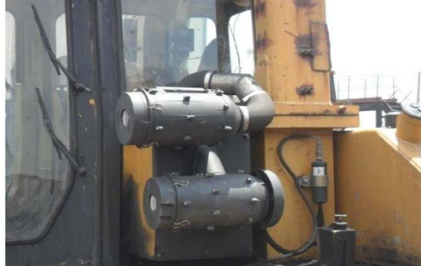
D11R Equipped with RESPA-CF/CFX Cab Air Quality System
