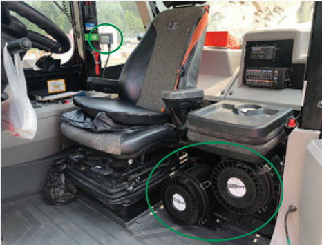
INSIDE CAB RECIRCULATION UNITS: RESPA FFX2 DUAL UNITS INSTALLED MONITOR: RESPA ADVISOR+
