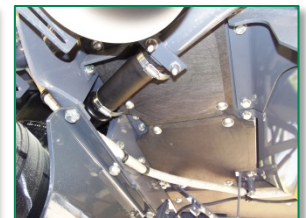
Factory Front Scavenger Line
