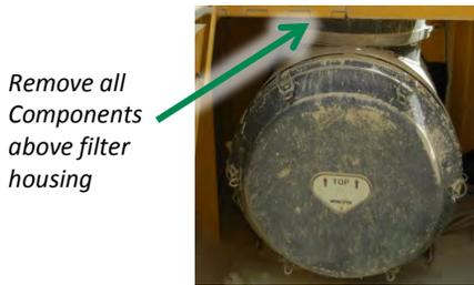
Remove all Components above filter housing
