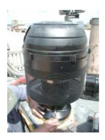
Install the scavenger <u>check valve</u> on the OPTIMAX scavenger port using a short piece of scavenger hose: then install the scavenger hose to the muffler.
