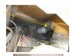
Remove plug from Muffler scavenger port.
