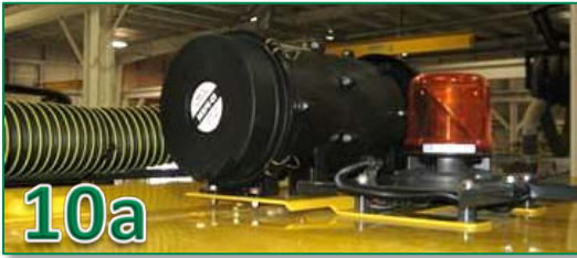
Wiring can be routed underneath beacon light bracket.
