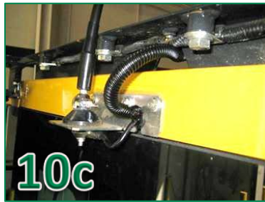
An existing grommet for the antennae can be used to enter the cab.
