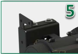
6. Using the existing recirculation box mounts, install the RESPA-FFX mounting plate as shown with M12x35 bolts (4), M12 washers (8), M12 lock washers (4), and M12 nuts (4).
