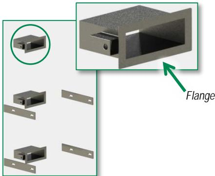
5. Apply sealant to face of duct.
