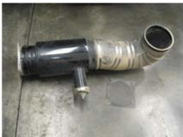
5. Clean the filter housing and inspect it for cracks, rusting or any other signs of damage. If you find any sign of damage replace the filter housing.
