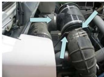
3. Remove the four screws as shown to remove the aluminum flange.
