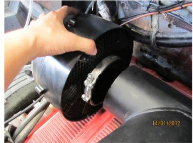
10. Make sure the ejections ports of the precleaners are facing down
