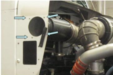
4. Remove the inlet piping and filter housing from the truck.
