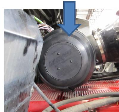
11. Install a new air filter and only change it when the filter minder reaches 25 in-H2O.
