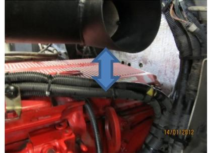
8. Tighten all the clamps to specification.
