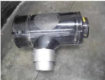
6. On the floor, clamp the AD0104 T-Adapter on the housing without the precleaners.
