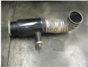
5. Clean the filter housing and inspect it for cracks, rusting or any other signs of damage. If you find any sign of damage replace the filter housing.
