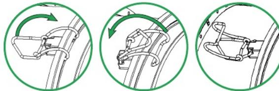
4. Install new filter element ensuring the ejection port orientation is correct and that the filter element end cap seats properly on the filter housing.
